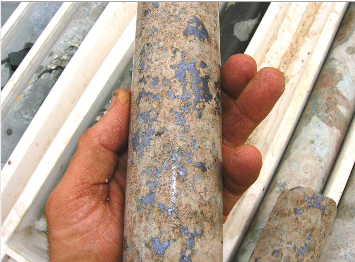
**Figure 1 – Coarse-grained molybdenite with accessory chalcopyrite.**
